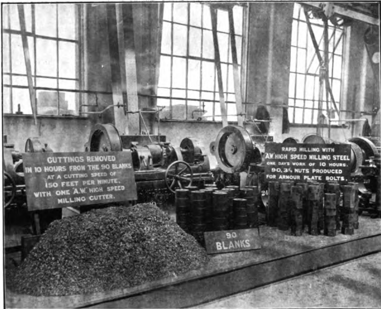
A. Making hexagon nuts from rolled bars with cutters of "A. W." high-speed steel. 90 nuts are produced in a day of 10 hours. Total weight of cuttings removed per day, 675 lbs. (Sir W. G. Armstrong, Whitworth & Co., Ltd., Manchester.)
